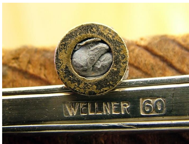
The Wellner mark together with a washer of 6.73 mm external diameter.
